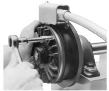
10. Reset the Autogap by pressing the armature toward the magnet or rotor.
