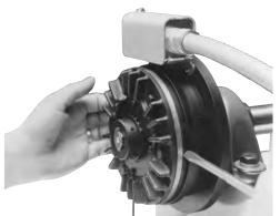
2. Remove hex head cap screws, washers and lock washers to loosen the armature segments from the cast iron carrier.
