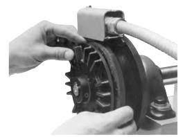
Attach the new friction material segments to the brake magnet or clutch rotor with the screws through the appropriate access holes. Apply one drop of Loctite (grade AA or equivalent) to each screw.
