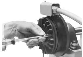
5. Lift out the worn friction material segments. Assure that the autogap plate, detent ring and spring remain in place on the clutch units during this step.
