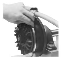
Attach the new armature segments to the cast iron carrier with hex head cap screws, lock washers and washers. Apply one drop of Loctite (grade AA or equivalent) to each screw. Tighten to the appropriate torque for your size unit.
