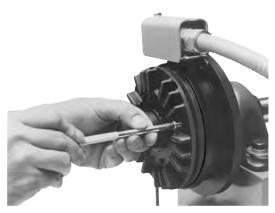
8. Insert the two new armature segments.
